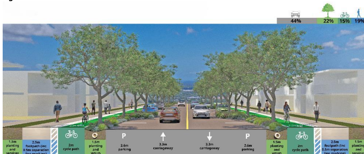
Figure 5: Cross section — 2 lane district collector
