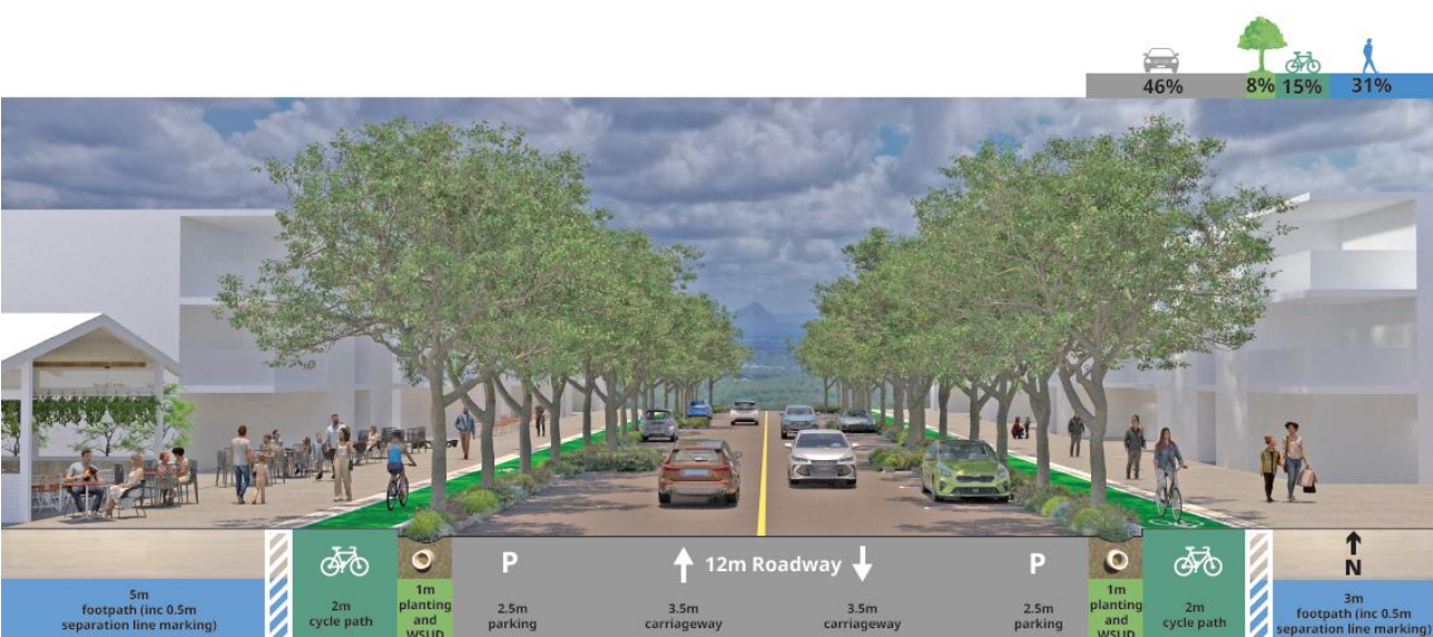
Figure 8: Cross section — Waraba Town Centre Main Street
