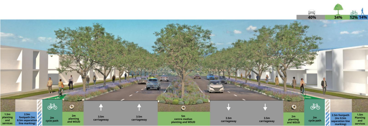
Figure 7: Cross section — 4 lane sub-arterial / arterial
